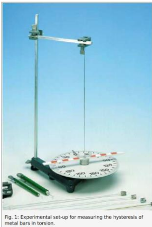
Fig. 1: Experimental set-up for measuring the hysteresis of metal bars in torsion.
